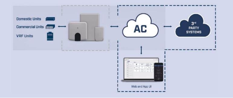
AC Cloud Control is an HVAC IoT solution that allows comfortable and intuitive control of air conditioners and heat pumps from a smartphone, tablet, smart watch or from a simple internet browser.
