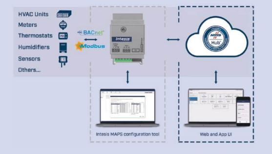
Intesis ST Cloud Control is an HMS cloud-based solution which enables easy monitoring and control of any BACnet or Modbus device by using our end user oriented App and web based dashboard.
