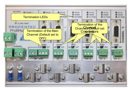
Fig. 15 - Termination Switches
