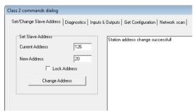
Fig. 21 - ProfiCaptain changes the address from 126 to 20
