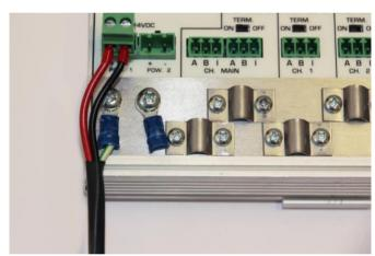
Fig. 12 - Connection to Ground Rail
