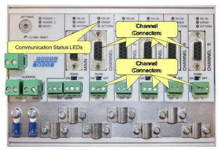
Fig. 14 - PROFIBUS DP spur connectors
