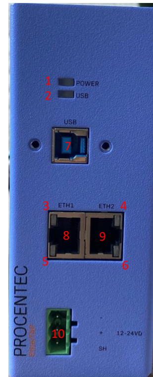
Figure 1: Identification of connections and LEDs for the 100 Mbit/s version
