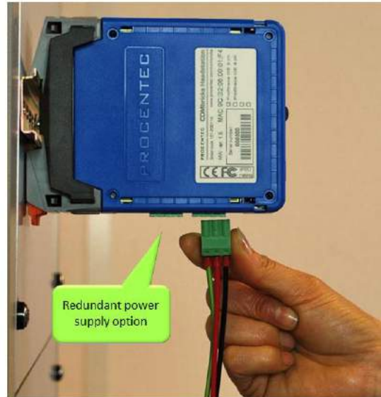
Powering the Head Station
