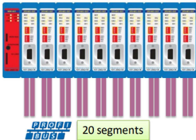
Figure 1 - 2 Channel repeater configuration example
